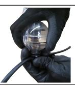
(d). Visually check the seal has not been trapped and is in good condition. In a clockwise twisting direction, lock and click the globe to the festoon cable.
