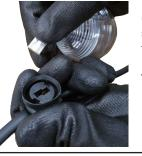
(b). The connection board should slide out of the festoon housing.
