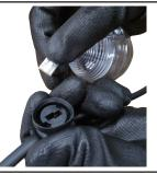
(b). Place connection board into festoon housing.
